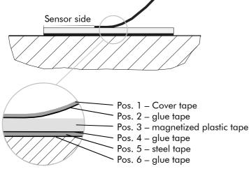
Picture 5: components of magnetic tape
