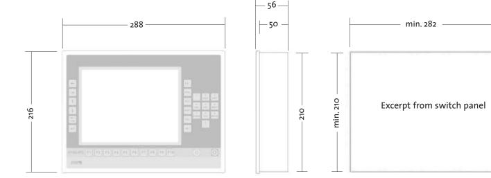
$\leftrightarrows$  Installation depth including connector and cable bend radius = 150 mm  $\because$  all dimensions in mm
