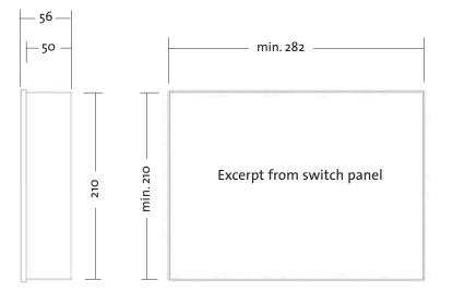
$\leftrightarrows$  Installation depth including connector and cable bend radius = 150 mm  $\leftrightarrows$  all dimensions in mm
