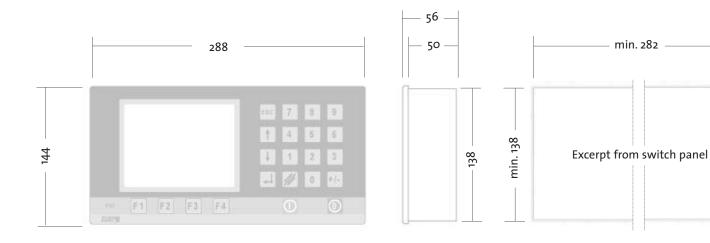
$\leftrightarrows$  Installation depth including connector and cable bend radius = 120 mm  $\leftrightarrows$  all dimensions in mm
