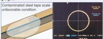
High insensitivity to contamination by use of a new scanning principle.
